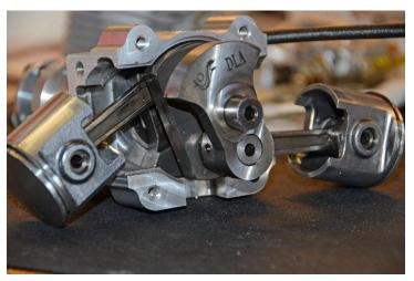
The rear half of the crankcase was removed to reveal the inside of the engine. Again, I was very pleased with the quality of machining DLA invested into the quality of this motor. The image to the left was slightly under-exposed to bring out the contrasting textures and surface details of each part. Yes! The "DLA" logo is etched into the rear of the crank, just above the rear bearing "button" in this view.
