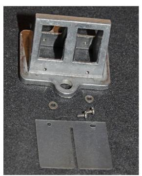
The reeds each have the appropriate amount of "bow". The screw-holes are very clean around the edges and free of any burrs. Unlike the "sheet-metal screw" counterpart, the machined screw renders a smooth hole with no burrs or ridge to distort or otherwise compromise integrity of the reed's ability to make full contact on the cage frame. Small washers increase the area of the screw head to reduce stress on the reeds and assure the reeds are held in place against the frame...
