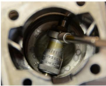
Both cylinders were "miced" for comparison to specifications and tolerance. Both cylinders were measured at the top of the stroke and bottom of the stroke. Two measurements were taken at 90 degrees apart to insure symmetry. Again, DLA came through with flying colors. None of the measurements showed any evidence of taper between the top and bottom of the stroke and the bore of both cylinders were within .005" of each other.
