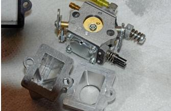
All three components are attached with two machine screws and sealed to the crankcase with a durable gasket. A machined aluminum flange fits in between the carb and reed valve assembly to provide adequate clearance. The reeds are attached with machine screws/washers to an aluminum reed valve "cage".
